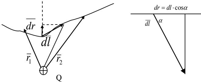
$$A_{12} = \int_{r_1}^{r_2} F dr = \int_{r_1}^{r_2} \frac{1}{4\pi\epsilon_0} \frac{qq_0}{r^2} dr = \frac{1}{4\pi\epsilon_0} qq_0 \left( \frac{1}{r_1} - \frac{1}{r_2} \right) \quad (4.2)$$
