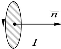
The diagram shows a circular current loop with a shaded interior. A small arrow on the left side of the loop indicates the direction of current flow. A horizontal arrow labeled  $\vec{n}$  points to the right from the center of the loop, representing the normal vector. Below the loop, the letter  $I$  is written. To the right of the diagram is the equation  $\mathbf{P}_m = IS\mathbf{n}$  and the label (11.1).
